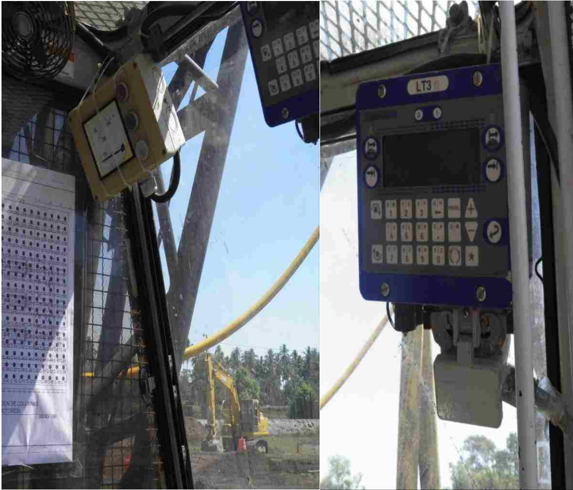
Figure 4.62. Jean Lutz LT3N parameter recorder and ampere meter
