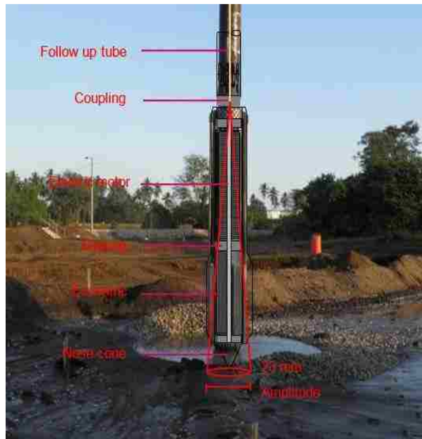
Figure 4.50. V23, Vibratroy probe schematic
